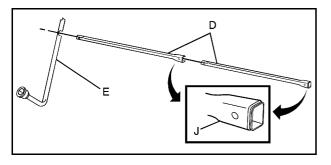
3. Assemble the two jack handle extensions (D) and wheel wrench (E) as shown.
